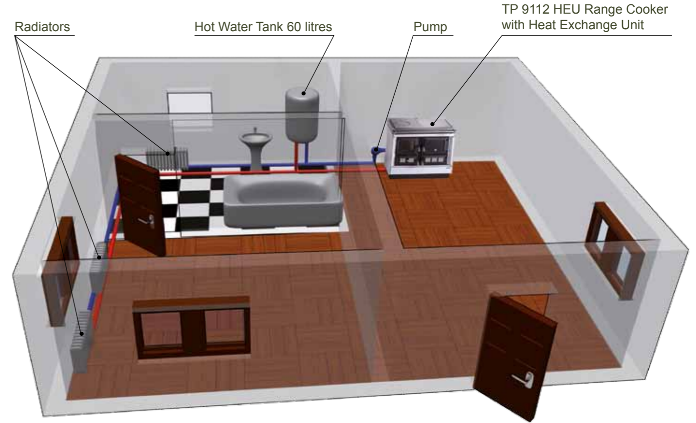
Solid fuel range cooker with oven for heating, cooking, baking and roasting and for connection to central heating hot water system
